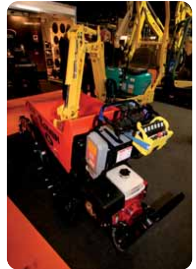
The 80 series tracked dumper can now be supplied with this radio remote control box.
